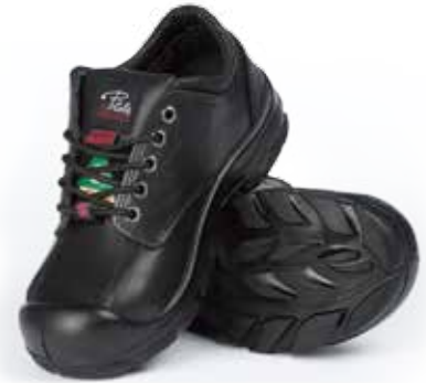
S557 LACED WORK SHOE : Double density P.U. outsole. Full grain leather upper. Cambrelle lining. Anti-bacterial and shock absorber removable insole. Inner heel wear protective reinforcement. Steel toe / steel plate CSA class 1. Dielectric approved. 560 g. / 1,2 lb per shoe. Color : black (N). Sizes : 5-12 (5,5 - 9,5).
