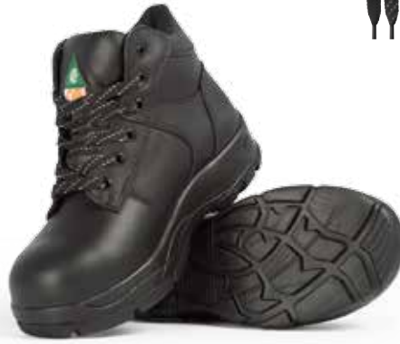
PF689 6" LACED WORK BOOT Ultra light EVA outsole. Full grain leather upper and tongue. Strong lining. 2 pairs of laces. Anti-bacterial and shock absorber removable insole. Kevlar midsole and steel toe CSA class 1. Dielectric approved. 570 g. / 1.3 lb per boot. Color : black (N). Sizes: 5 - 11 (6.5 - 8.5).
